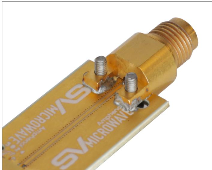
**Consequence:** This small rotation can eventually lead to damage of the solder joint. In extreme cases this can end in de-laminated traces or twisted solderwire.
